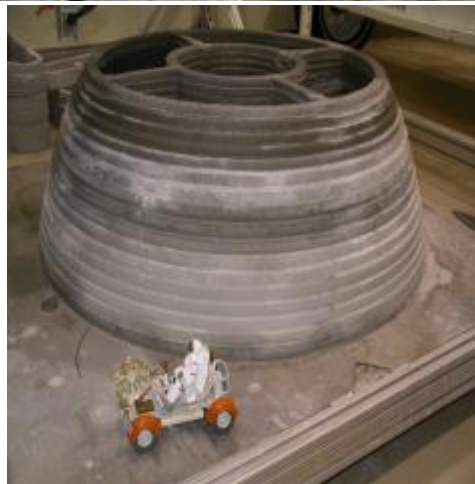
Complex Tool Path Development Allows Interior Walls
