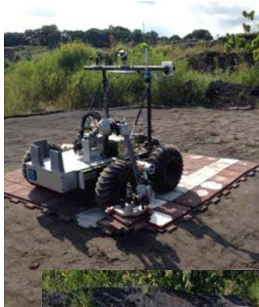
Robotic Paver Deployment Mechanism on PISCES Rover in Hawaii
